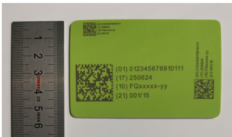
Example of laser engraving sizes on silicone (with a QR Code to scan to test its legibility).
